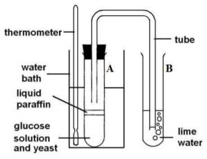
The gas produced in tube **A** passed through the delivery tube and formed bubbles in lime water in **B**.
